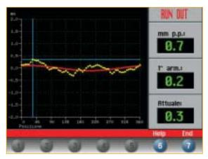
Eccentricity measuring system (1<sup>st</sup> Harmonic and Peak to Peak) with Sonar (option).
