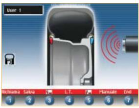
Automatic wheel width measurement with CEMB patented sonar system (option).
