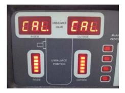
2. CLOSE THE HOOD AND PRESS THE START KEY. (THE MACHINE WILL SPIN THROUGH A COMPLETE CYCLE FOR AROUND 20 SECONDS AND THEN COME TO A COMPLETE STOP.)
