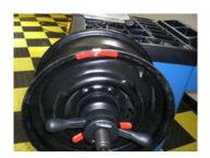
4. CLOSE THE HOOD AND PRESS THE START KEY. (THE MACHINE WILL SPIN THROUGH ANOTHER COMPLETE CYCLE FOR AROUND 20 SECONDS AND THEN COME TO A COMPLETE STOP.)
