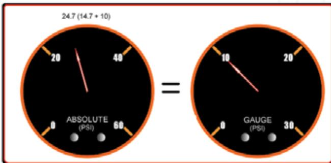
In determining Pressure Ratio, the Absolute Pressure at the compressor inlet (P2c) is often LESS than the Ambient Pressure, especially at high load. Why is this? Any restriction (caused by the air filter or restrictive ducting) will result in a "depression," or pressure loss, upstream of the compressor that needs to be
