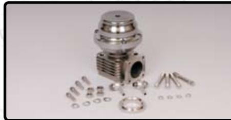
External wastegates are added to the exhaust plumbing on the exhaust manifold or header. The advantage of external wastegates is that the bypassed flow can be reintroduced into the exhaust stream further downstream of the turbine. This improves the turbine's performance. On racing applications, this wastegated exhaust flow can be vented directly to atmosphere.
