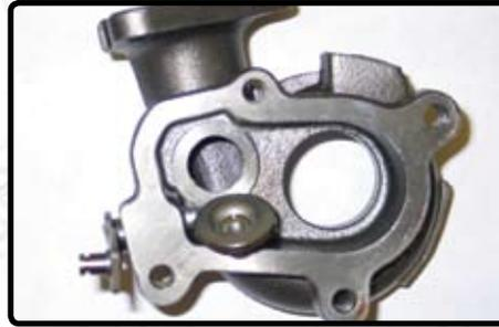
Internal wastegates are built into the turbine housing and consist of a "flapper" valve, crank arm, rod end, and pneumatic actuator. It is important to connect this actuator only to boost pressure since it is not designed to handle vacuum and as such should not be referenced to an intake manifold.
