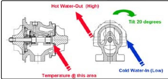
Negative degrees: water outlet of center housing is lower than water inlet
