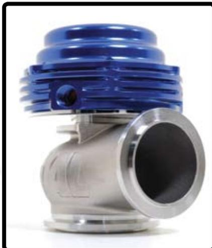
All TiAL wastegate assemblies are constructed with stainless steel valves and valve bodies. Actuator housings are CNC machined billet aluminum, with an optimal actuator to valve ratio or 2.2:1 for maximum flow capacity. The units are
