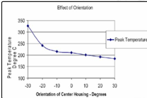
For best results, set the orientation of the center housing to 20°. Significant damage to the turbo can occur from improper water line setups.
